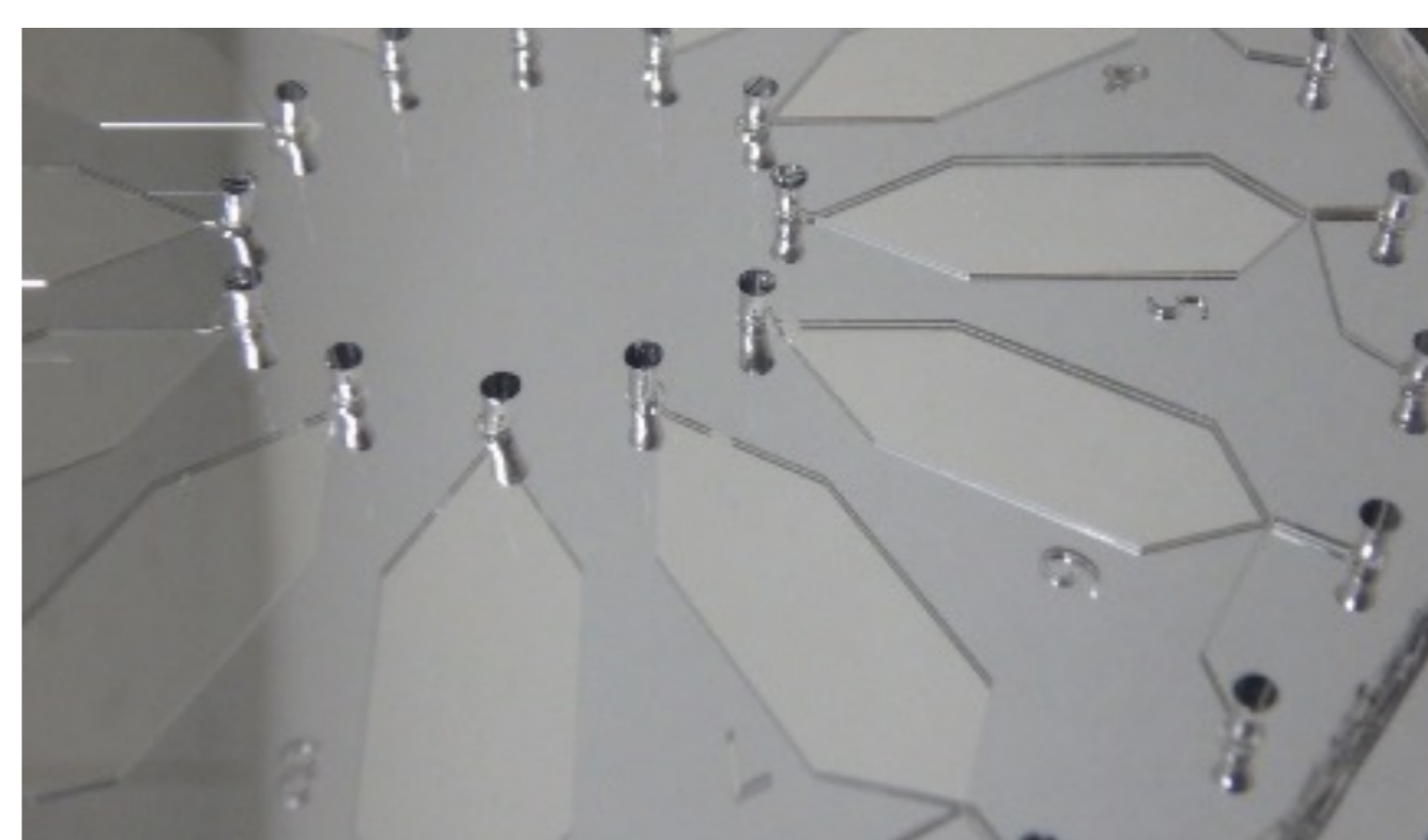
Microfluidic device for DNA purification
