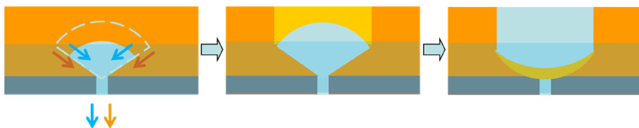
Soil below the ground water level flows with water through the hole. A cavity can expand. Ceiling of the cavity reaches near the ground surface. Collapse of the soil above the cavity
