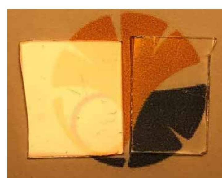
Reflection image of glass before (left) and after (right) surface treatment
