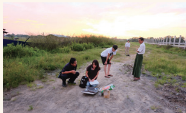
Measuring of microtremor to evaluate ground condition in Yangon City
