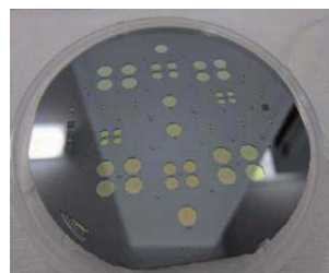
100mm wafer with 8 layers Bragg mirror membranes
