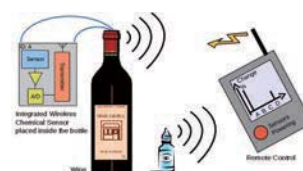
Principle of the system. A remote control powers on the integrated chemical sensors placed inside the container. The sensors transmit their answer in a wireless way.
