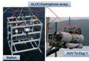
Instruments used at the sea trial. Left: Seafloor station Right: AUV Tri-Dog 1
