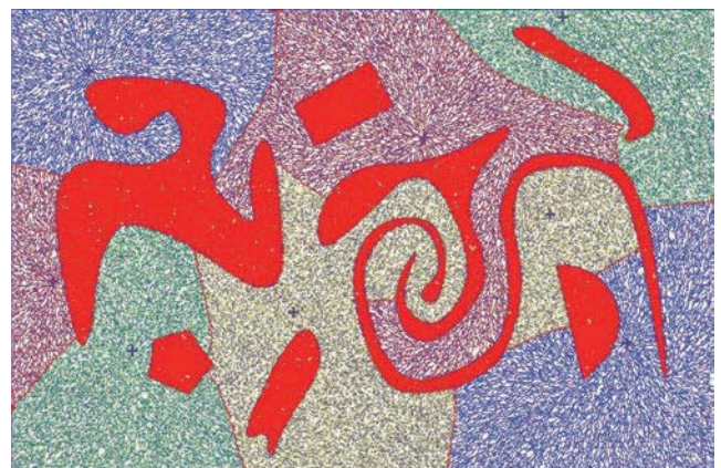
Voronoi diagram with eight strange shape obstacles by eight generators
