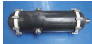
Hemispherical end caps and cylinder made of silicon nitride ceramics, and connection rings made of zircon ceramics (Operational water depth= 11,000m, safety factor= 2)
