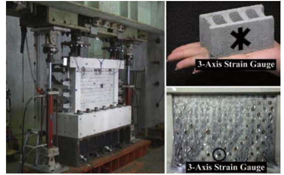
Test setup (left), 1/4 scaled concrete block (top-right), URM Wall with 3-axis strain gauges (bottom-right)
