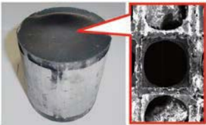
Automotive catalytic converter. Precious metal particles are distributed in oxide mixtures.
