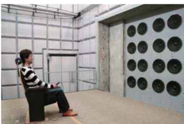
System of hearing subjective test on low-frequency noise
