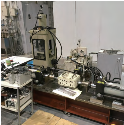
Servo-type apparatus of tube hydroforming process
