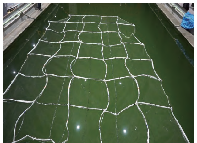
Water tank testing of a hose net in IIS Ocean Engineering Basin
