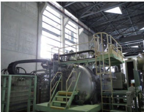
Apparatus of electron beam melting
