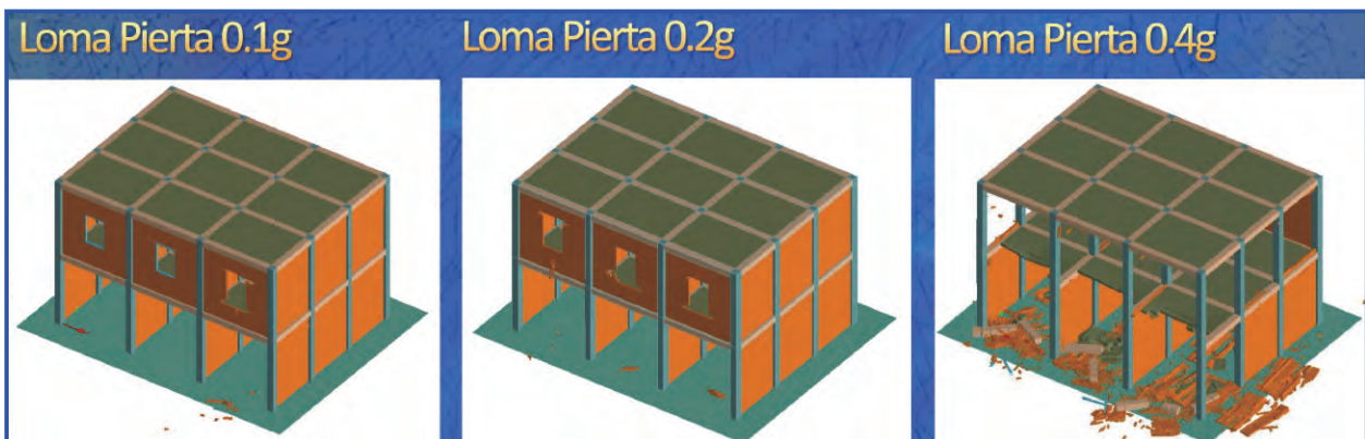
In AEM, simulated object is regarded as the groups of elements. Each element is connected by normal and shear springs.
