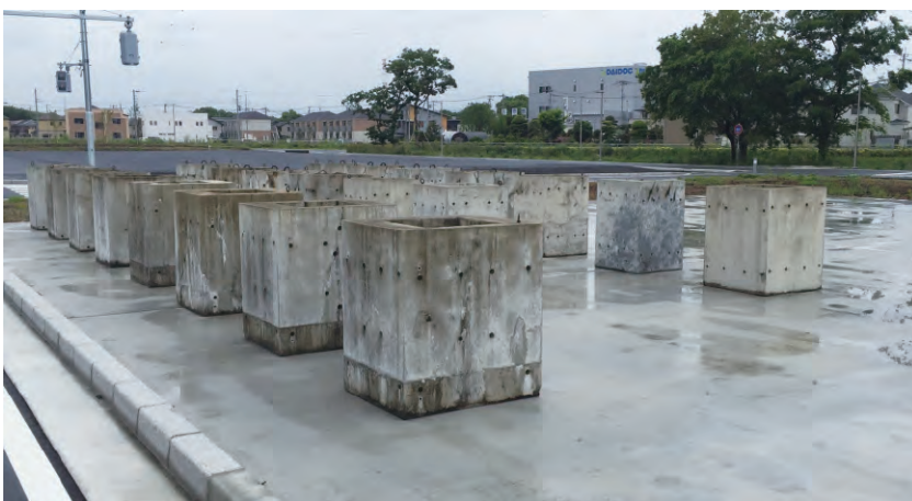
Specimens of developed self-healing concrete
