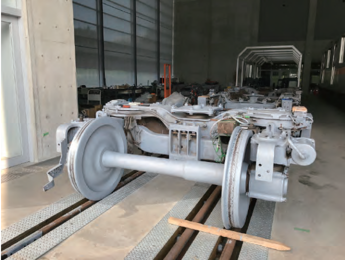
Experimental bogie for the detection of the irregularity on the rail
