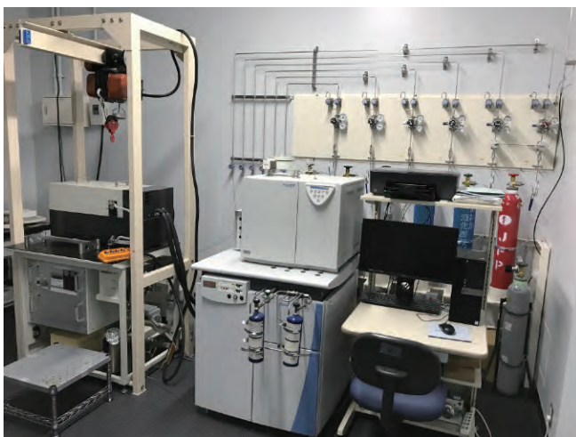
Mass spectrometer used for analyzing stable water isotope ratio
