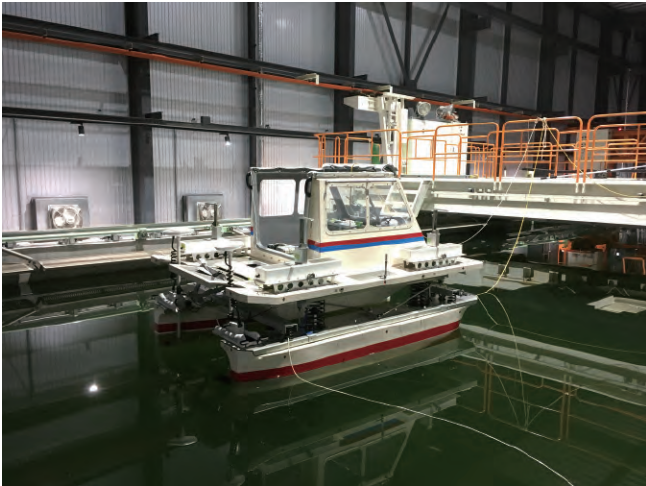
Water tank testing of WHzer (Wave Harmonizer) 8 in IIS Ocean Engineering Basin
