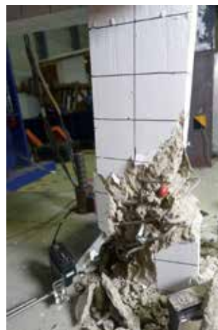
津波漂流船舶の柱衝突実験 Impact of tsunami driven vessel on dynamic behavior of RC columns
