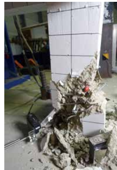
津波漂流船舶の柱衝突実験 Impact of tsunami driven vessel on dynamic behavior of RC columns
