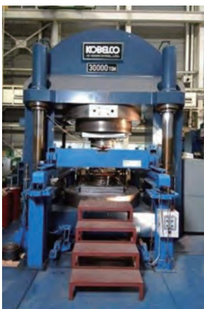
Belt-type high pressure apparatus, synthesis conditions, and variety functions of boron nitride crystals
