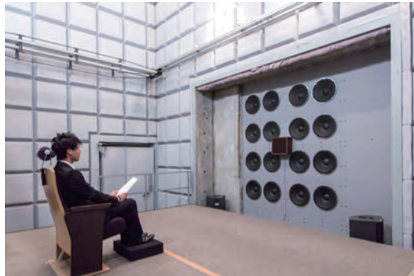
半無響室における低周波騒音の聴感評価実験 Psycho-acoustical experiment on low frequency noise in hemi-anechoic room
