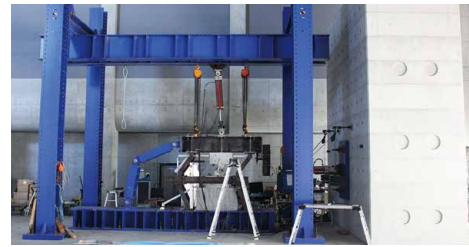
静的载荷関連設備および反力壁 Static loading related facilities and reaction wall
