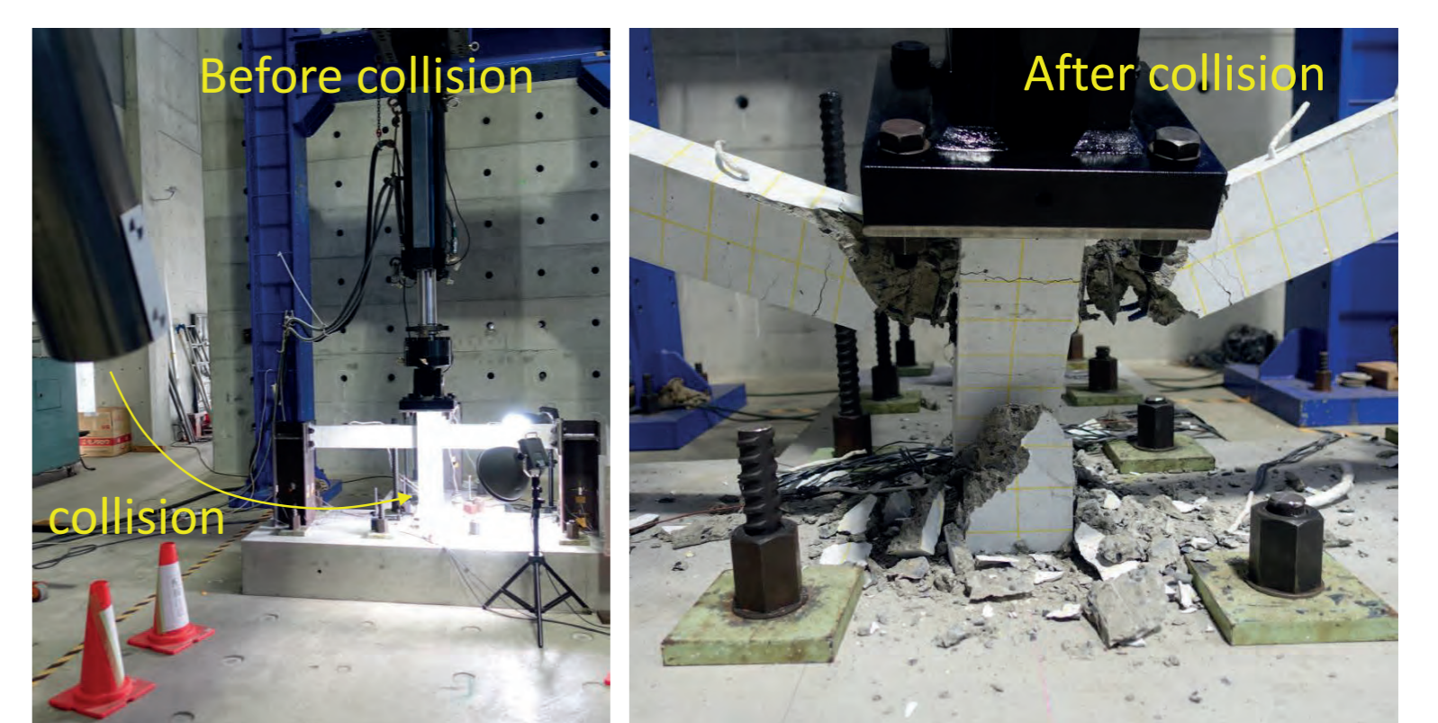
Collision Test and Collapse of Reinforced Concrete Frame
