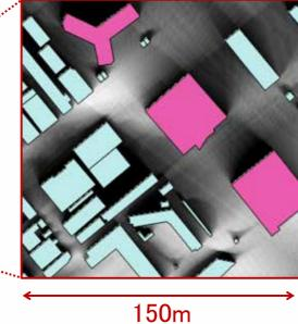
The shadows cast by high-rise buildings, can sometimes be over 1 km long and affect a wide area. In this study, a system with more than 4,000 building data and 160,000 candidate points is implemented to analyze composite shadows.
