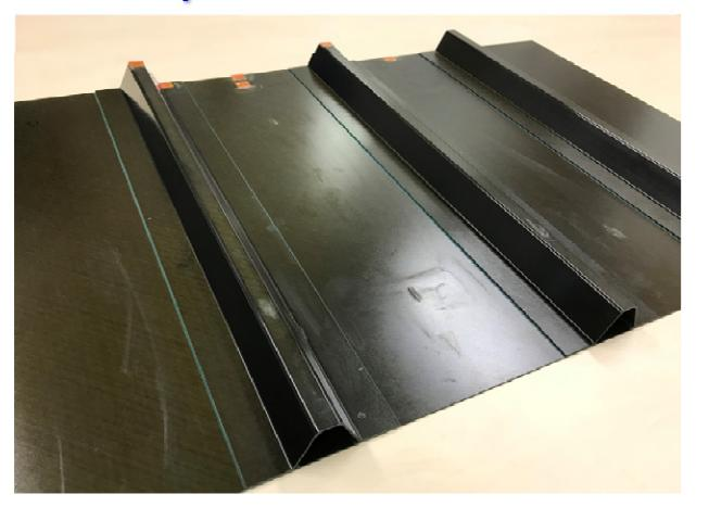
CFRP stiffened panel
