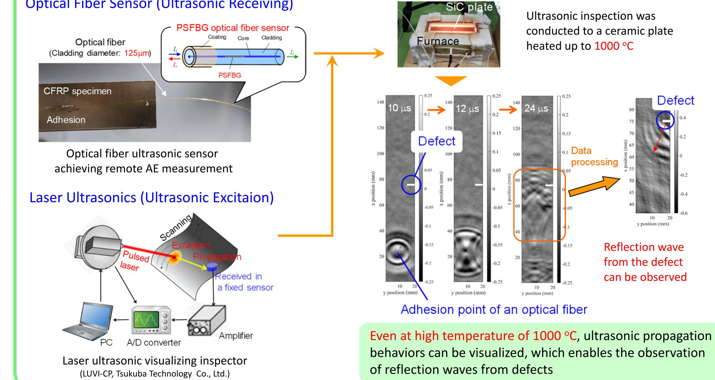
Ultrasonic inspection was conducted to a ceramic plate heated up to 1000 °C
