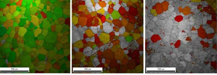
Superposed image quality (IQ) in greyscale and grain orientation spread (GOS) maps of the polished Sn-1.0wt%Bi alloy one hour after polishing under different pressures.
