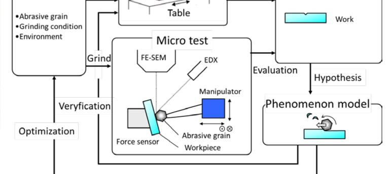
Flow of optimal grinding wheel development by single grain cutting test
