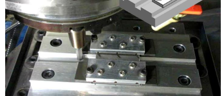
Evaluation test of cutting tools for CFRP
