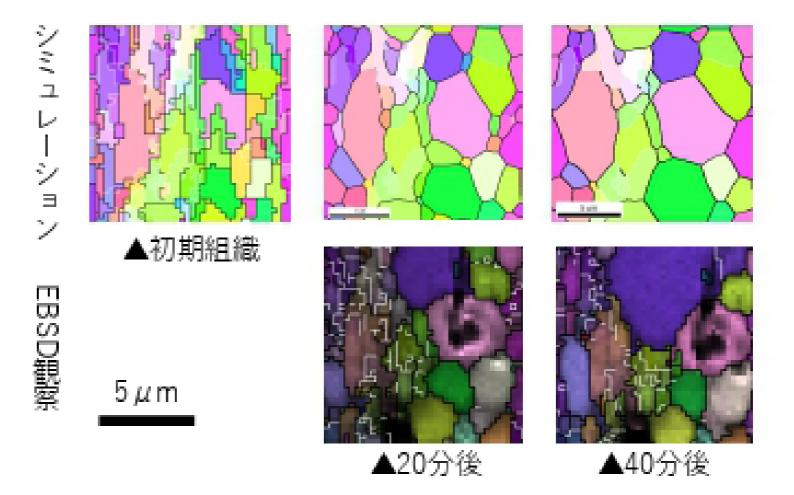
recrystallization behavior of industrial pure aluminum. In this example, grain structures are obtained during heat-treatment using EBSD analysis and a phase-field simulation based on subgrain growth model is applied. The precipitation and strain energy stored in each grains are estimated.
