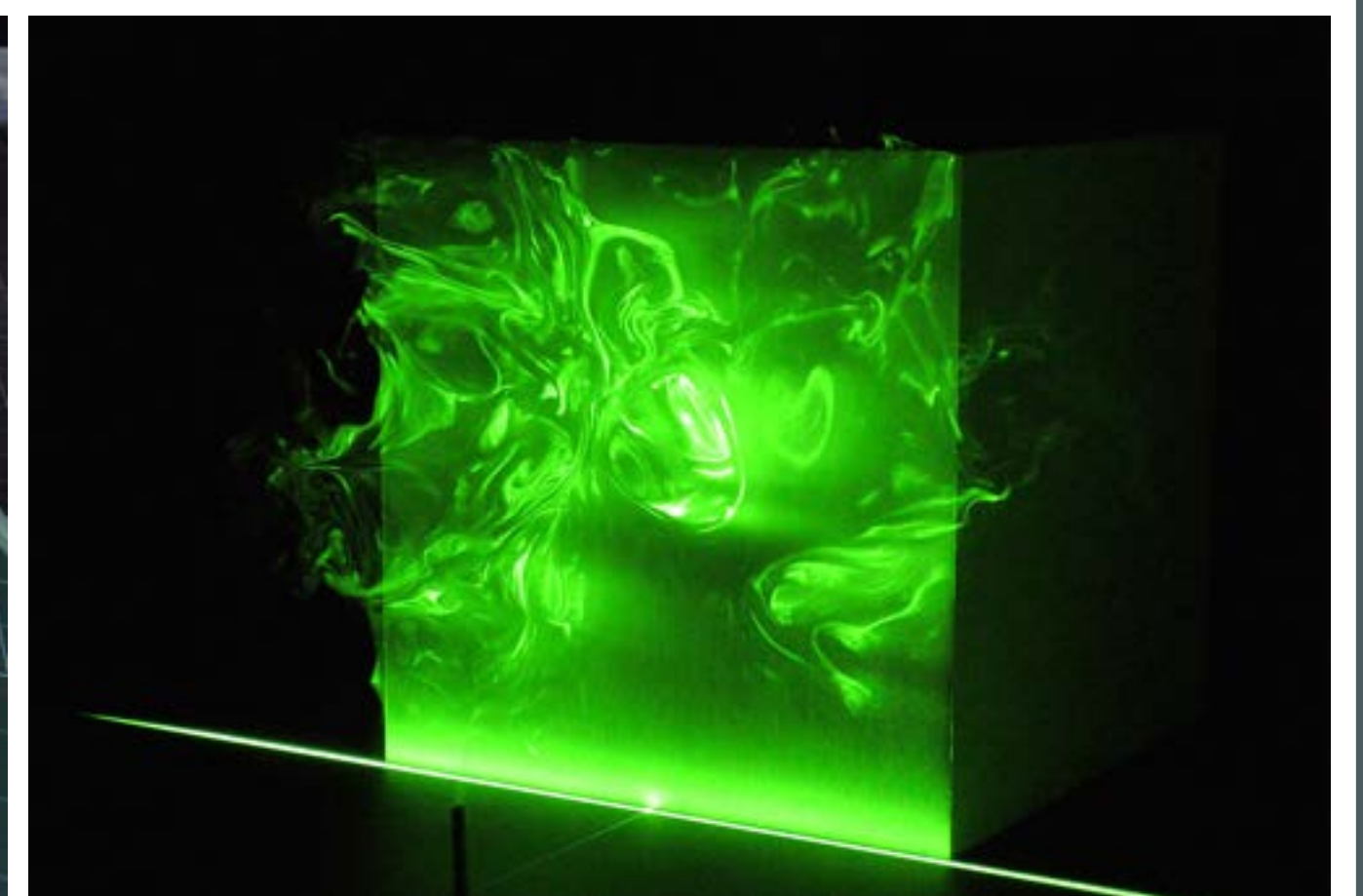
Visualization of pollutant dispersion in wind tunnel
