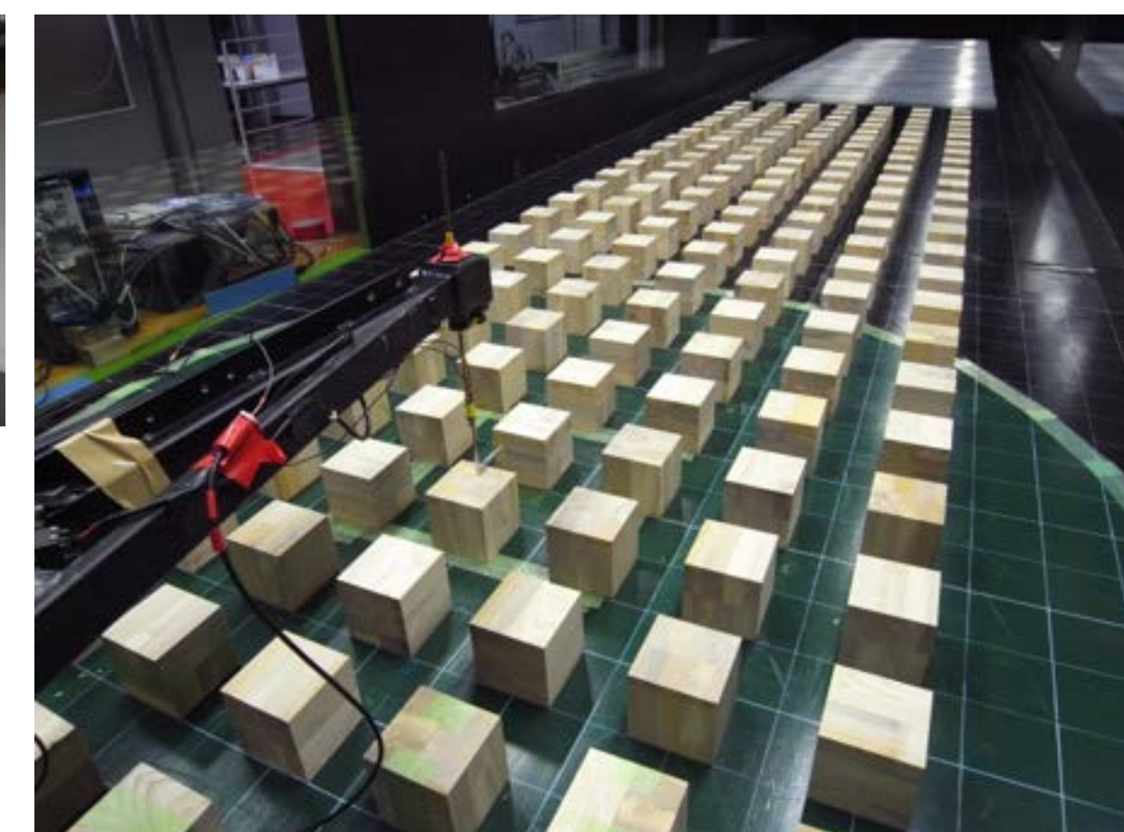
Wind tunnel experiment of city airflow
