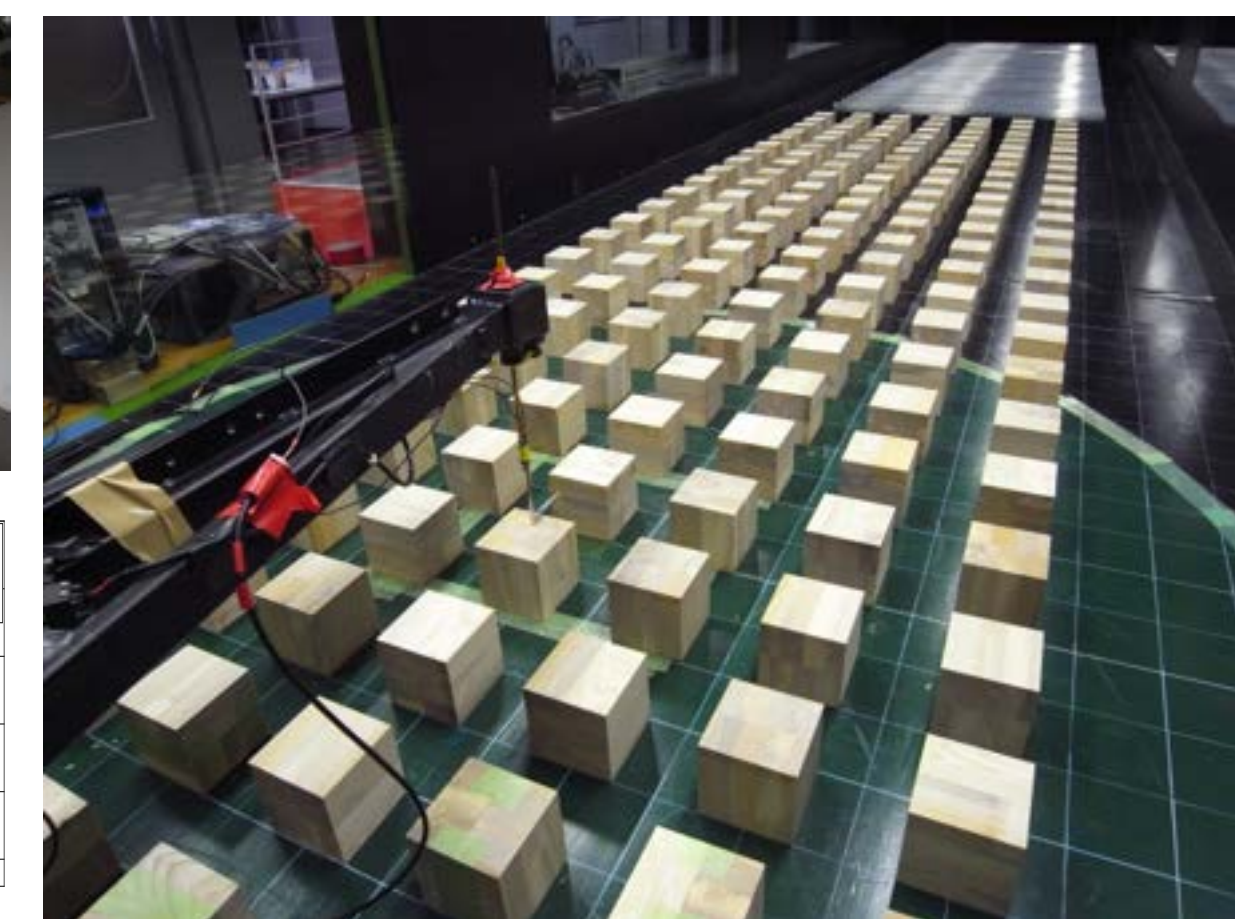
Wind tunnel experiment of city airflow
