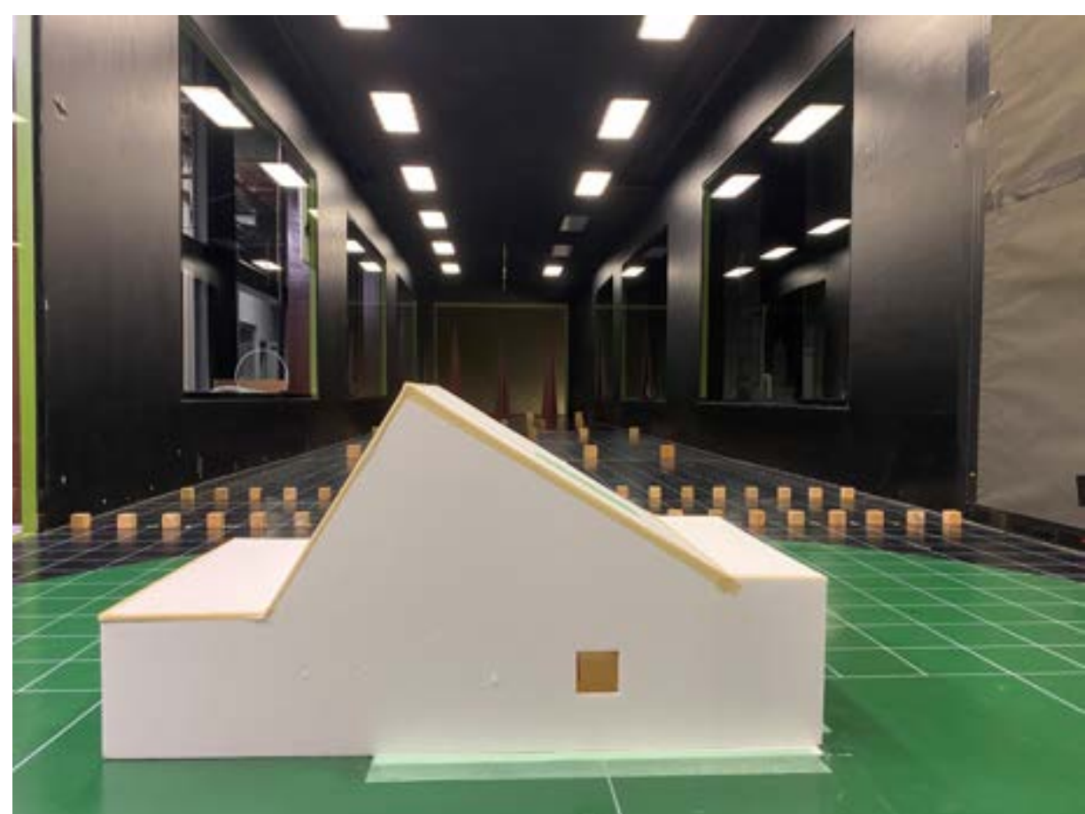
Experimental house natural ventilation evaluation using 3 methods (field measurement, wind tunnel experiment, CFD simulation)
