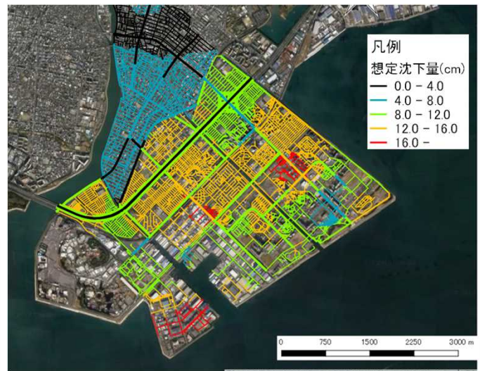
Newly-developed liquefaction hazard map for road network in Urayasu City
