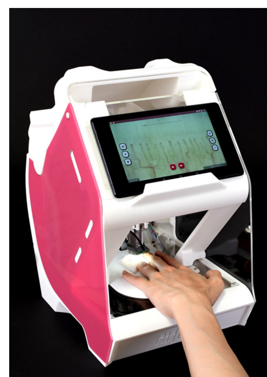
Developed observation system for the nailfold capillary
