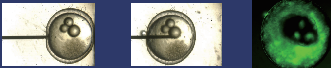
Injecting protective agents into a fish egg by immobile needle using electro-piercing (left: Before the electric pulse, center: after the pulse, right: after freeze-thawing; dark part depicts embryonic cells)
