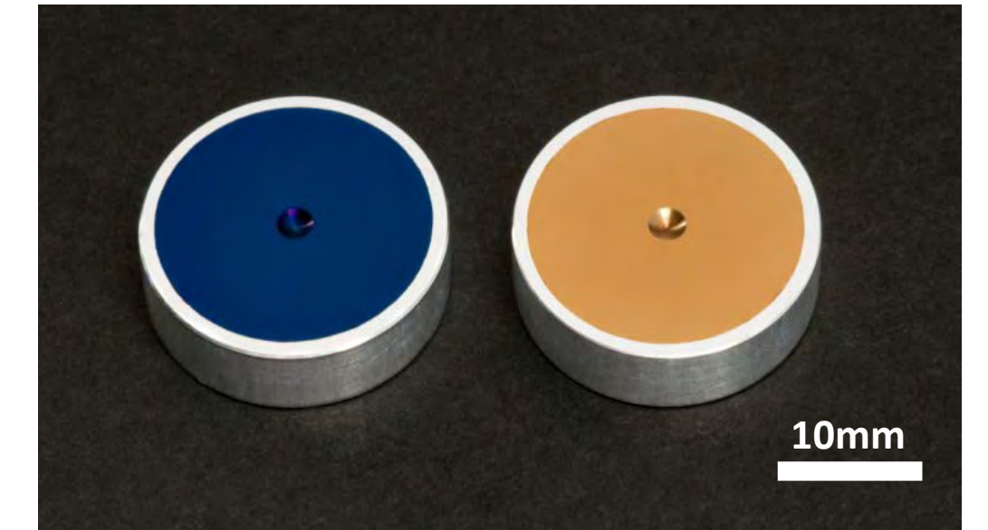
Aluminum alloy parts coated with DLC. Differences in color are caused by interference depending on the film thickness. This indicates that DLC is transparent in the visible light region.
