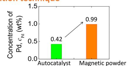
⇒ PGMs were concentrated by magnetic separation after Ni plating.
