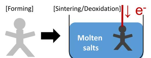
High-quality Ti products can be produced by sintering and deoxidation in molten salt
