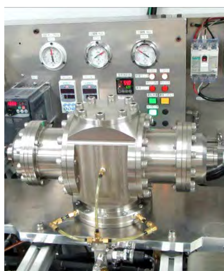
Two phase expander & demonstration unit for trilateral cycle
