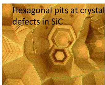
Growth interface during solution growth of SiC at 1400°C
