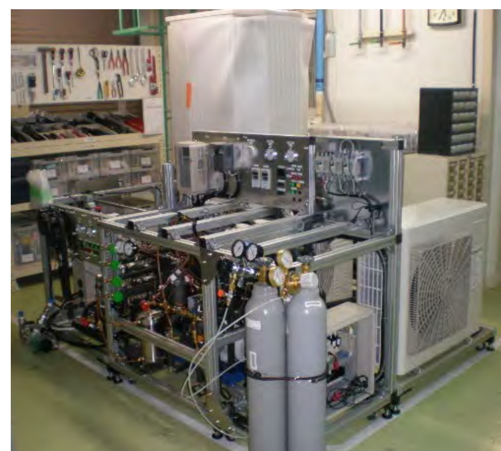
Two phase expander & demonstration unit for trilateral cycle
