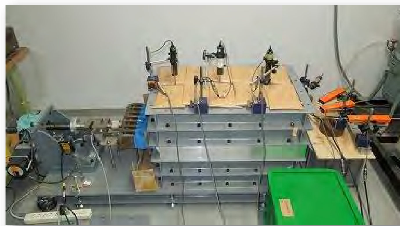
Pull-out test and shaking table model test on newly developed Geo-cell reinforced retaining wall
