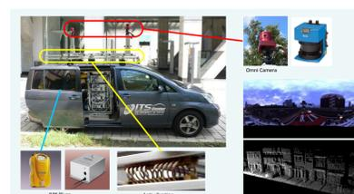
Using omnidirectional cameras, laser range scanner, etc., 3D geometry and photometric attributes of surrounding structures such as buildings and roads are collected
