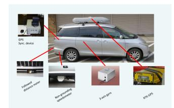
Precise measurement of location, speed, acceleration, and direction of the experimental vehicle itself with relative positioning of the following vehicle
