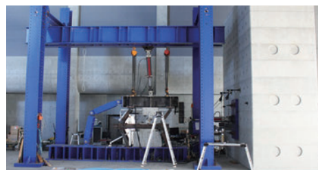
静的载荷関連設備および反力壁 Static loading related facilities and reaction wall
