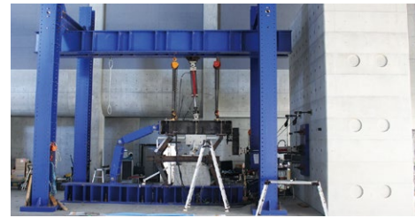
静的載荷関連設備および反力壁 Static loading related facilities and reaction wall
