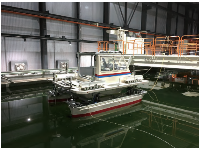
Water tank testing of WHzer (Wave Harmonizer) in IIS Ocean Engineering Basin
