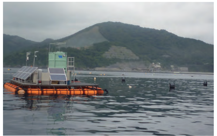
Prototype of a controllable depth cage installed in Onagawa Bay
