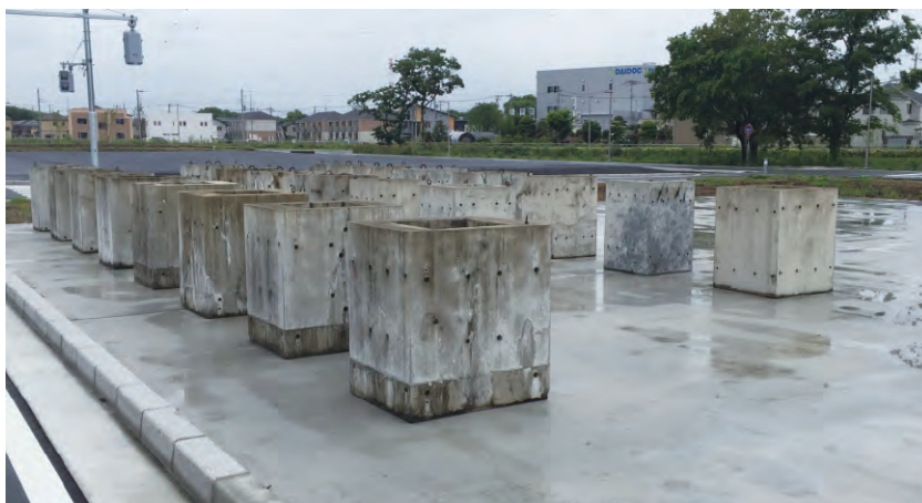
Exposure test of developed self-healing concrete
