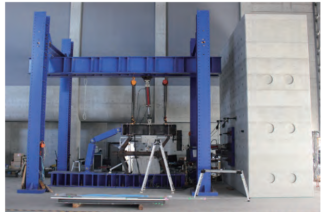
Static loading related facilities and reaction wall
