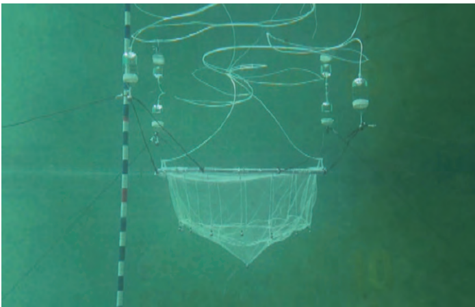
Water tank testing of the performance of a controllable depth cage
