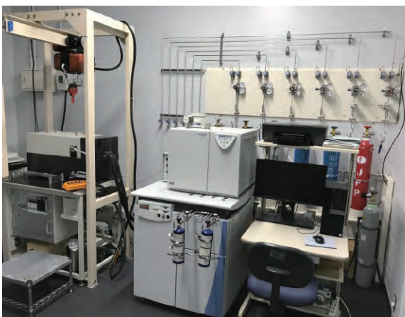
Mass spectrometer used for analyzing stable water isotope ratio
