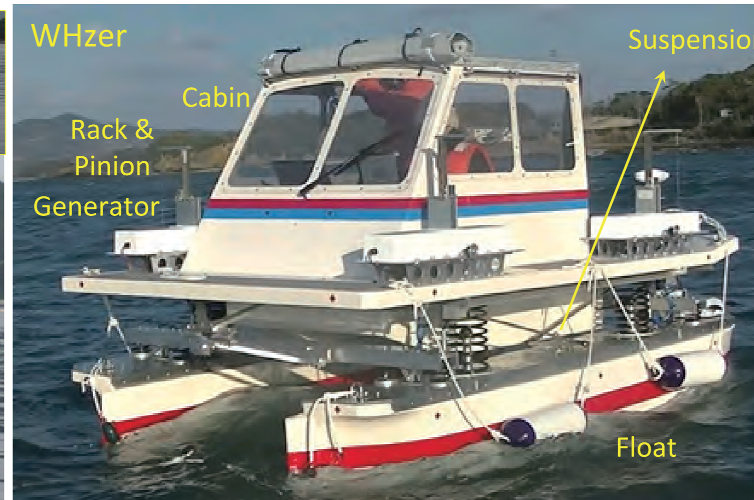
Wave Harmonizer Motion-controlled ship with wave energy harvester
