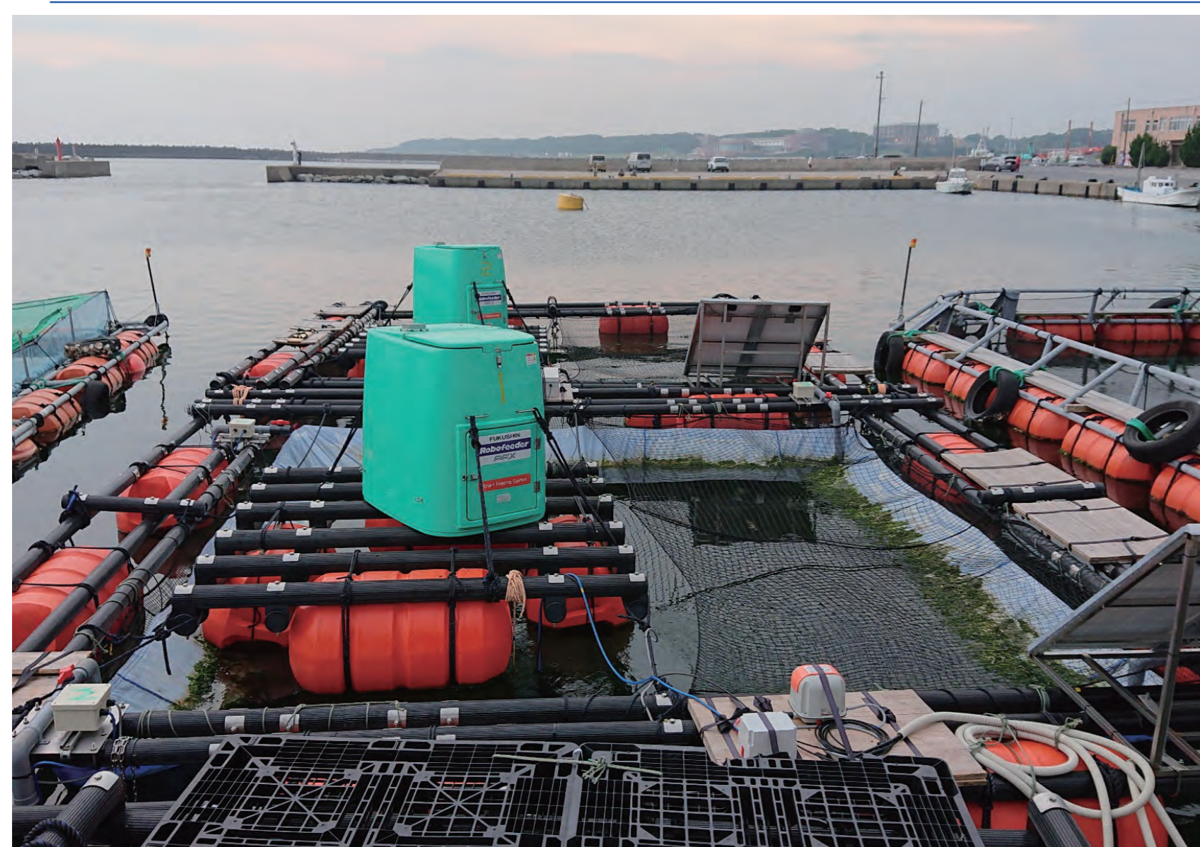
Marine Semi-closed Circulation Aquaculture System Robust aquaculture against high water temperature and red tide
