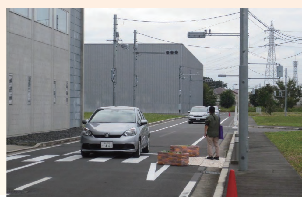
Field experiment of "bulb-out" at midblock crosswalk
