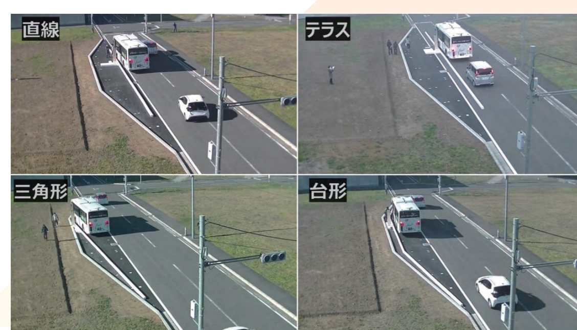
Field experiment comparing geometric designs around a bus stop
