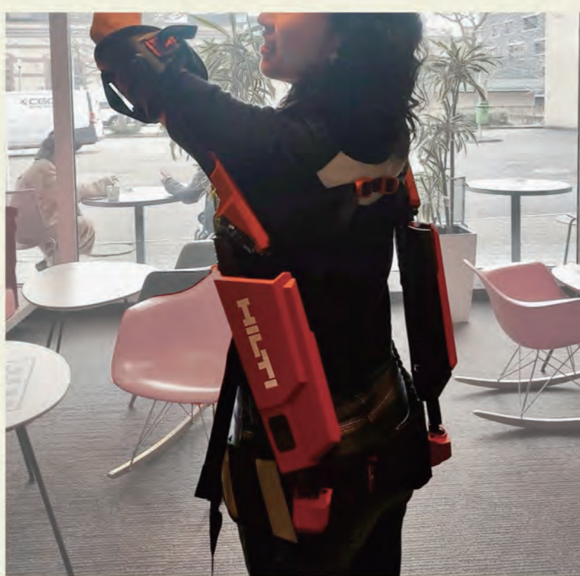
Exoskeleton to assist the construction work. [2025]
