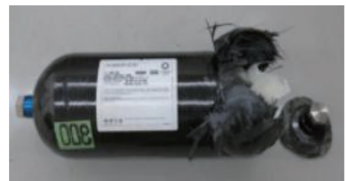
Validation of simulation by tank burst test
