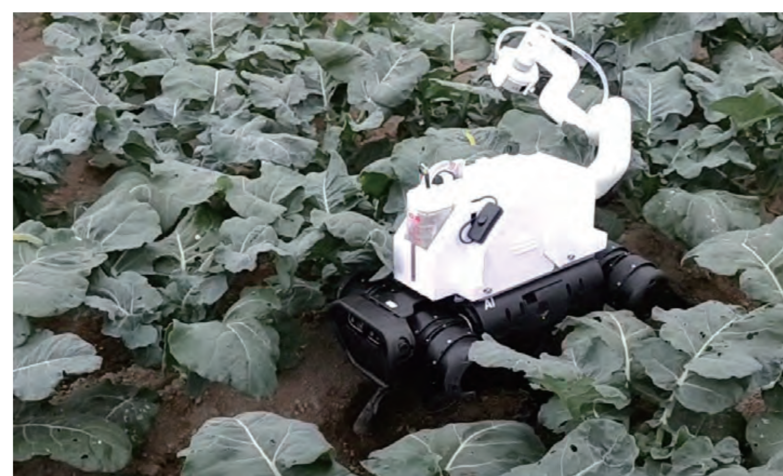
Agricultural support robot (pest detection, pesticide spraying)
