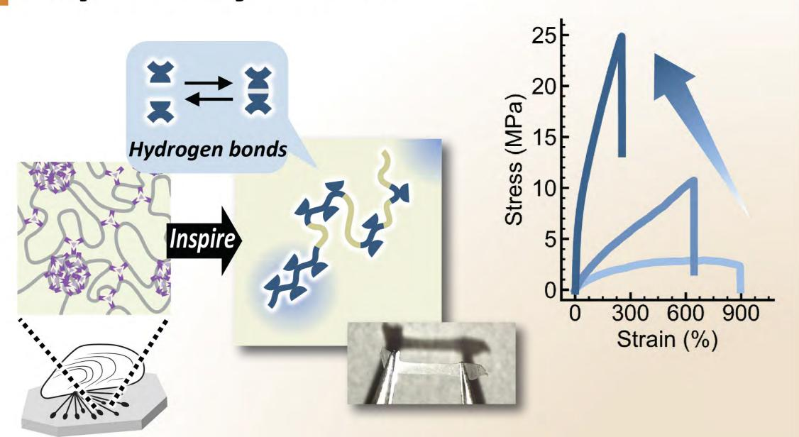
Mussels have a string-like tough organ called byssus to fix themselves to rocks. Inspired by the multiphase structure formed by dynamic crosslinks in byssus, we developed a new material with high mechanical toughness.
