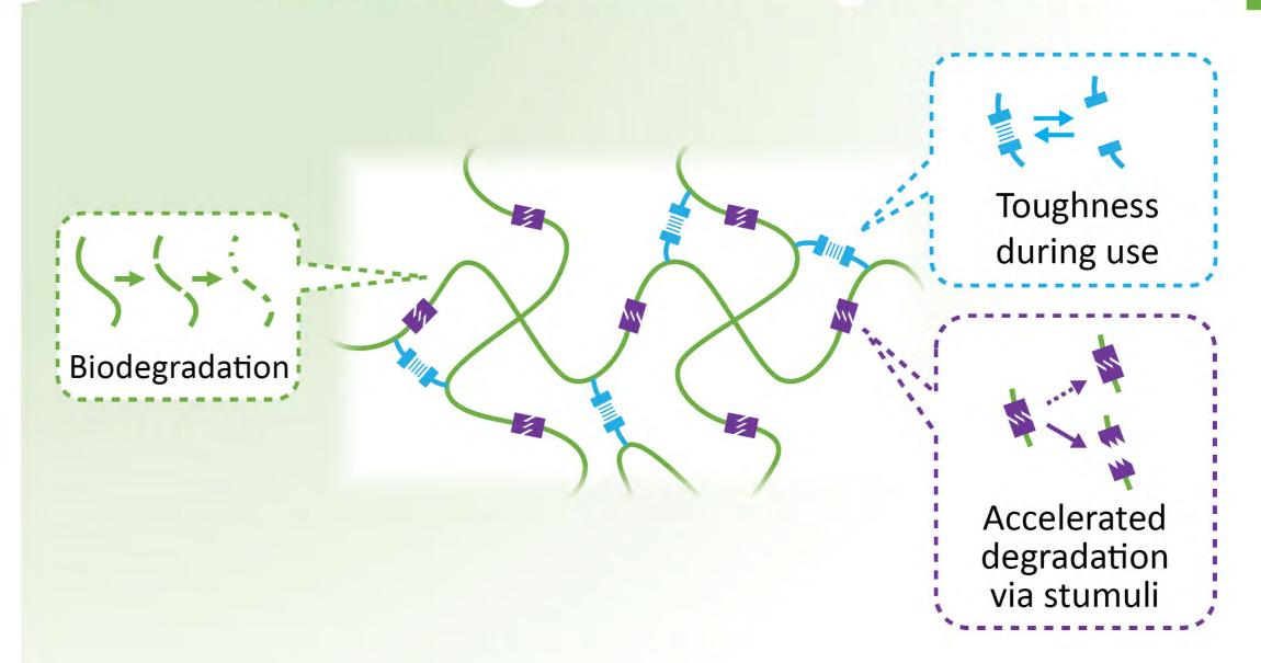
To tackle the global issue of plastic wastes, polymers that can degrade in environment are highly anticipated. We are developing polymer materials that keeps good toughness during use and can degrade rapidly by external stimuli in nature.
