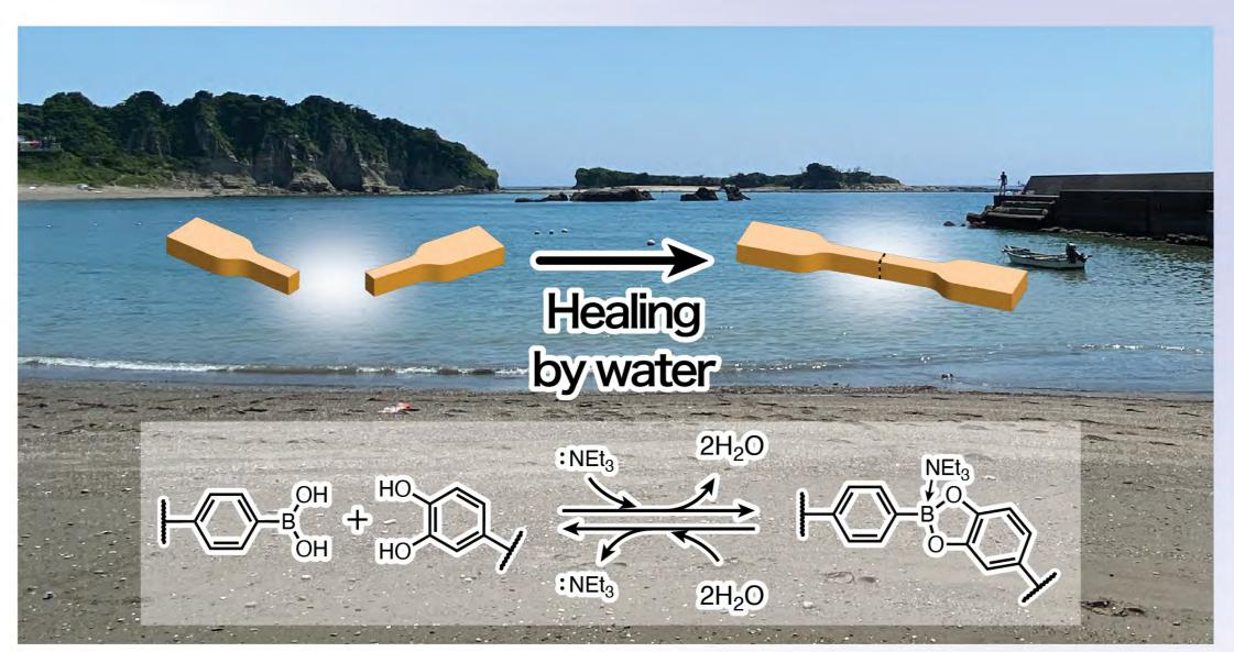
Water is a very attractive stimulus source that exist everywhere on earth. We have developed polymers that heals with the assistance of water. They absorb small amount of water molecules in air and in seawater, which heals the damage of the polymers with the collaboration of boronate esters in the polymer chain.
