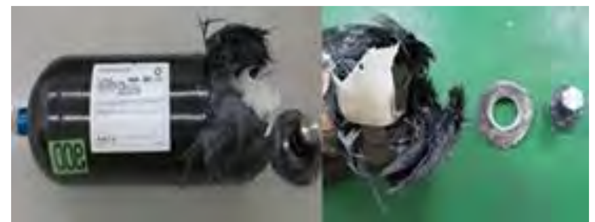
Validation of simulation by tank burst test
