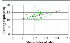
Relationship between the edge shape of a cutting blade and its cutting performance.
