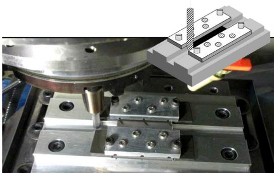
Evaluation test of cutting tools for CFRP
