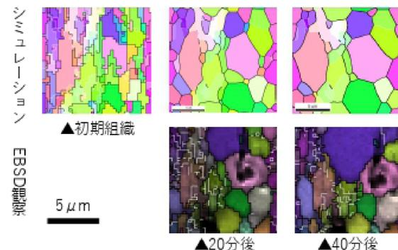
Data assimilation has been applied to clarify the mechanism controlling the recrystallization behavior of industrial pure aluminum. In this example, grain structures are obtained during heat-treatment using EBSD analysis and a phase-field simulation based on subgrain growth model is applied. The precipitation and strain energy stored in each grains are estimated.
