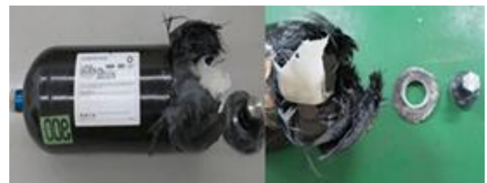
Validation of simulation by tank burst test
