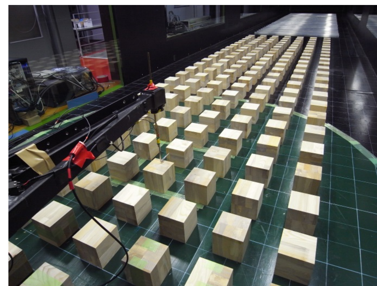
Wind tunnel experiment of city airflow
