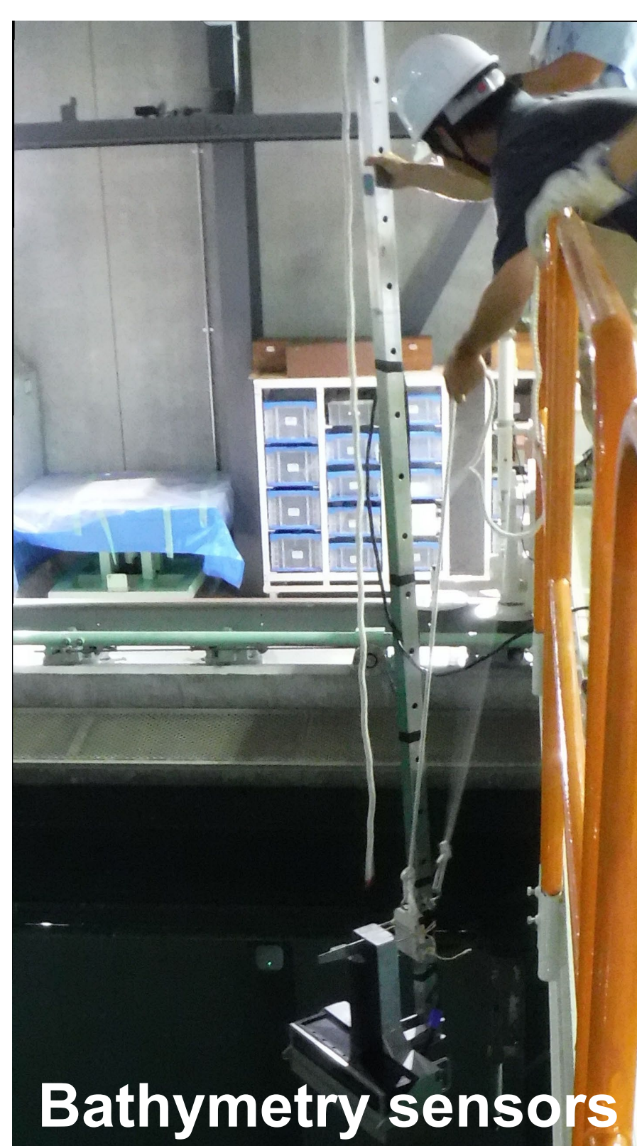
Fig4: Experiment of Multibeam-echosounder
