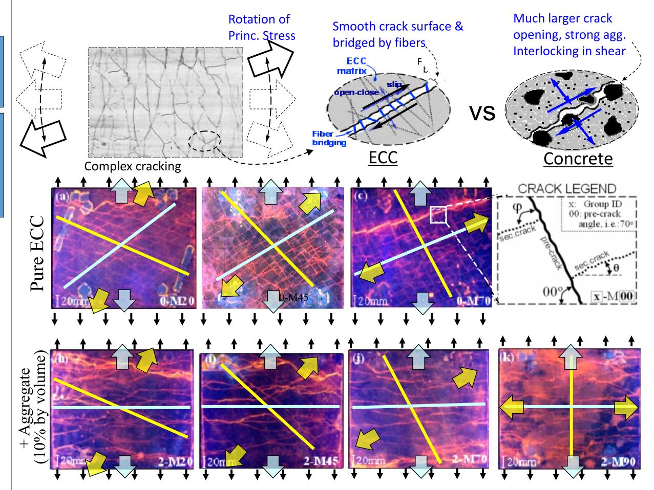
Control of cracking direction of HPFRCC
