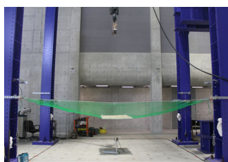
Real-scale tests of the safety net
