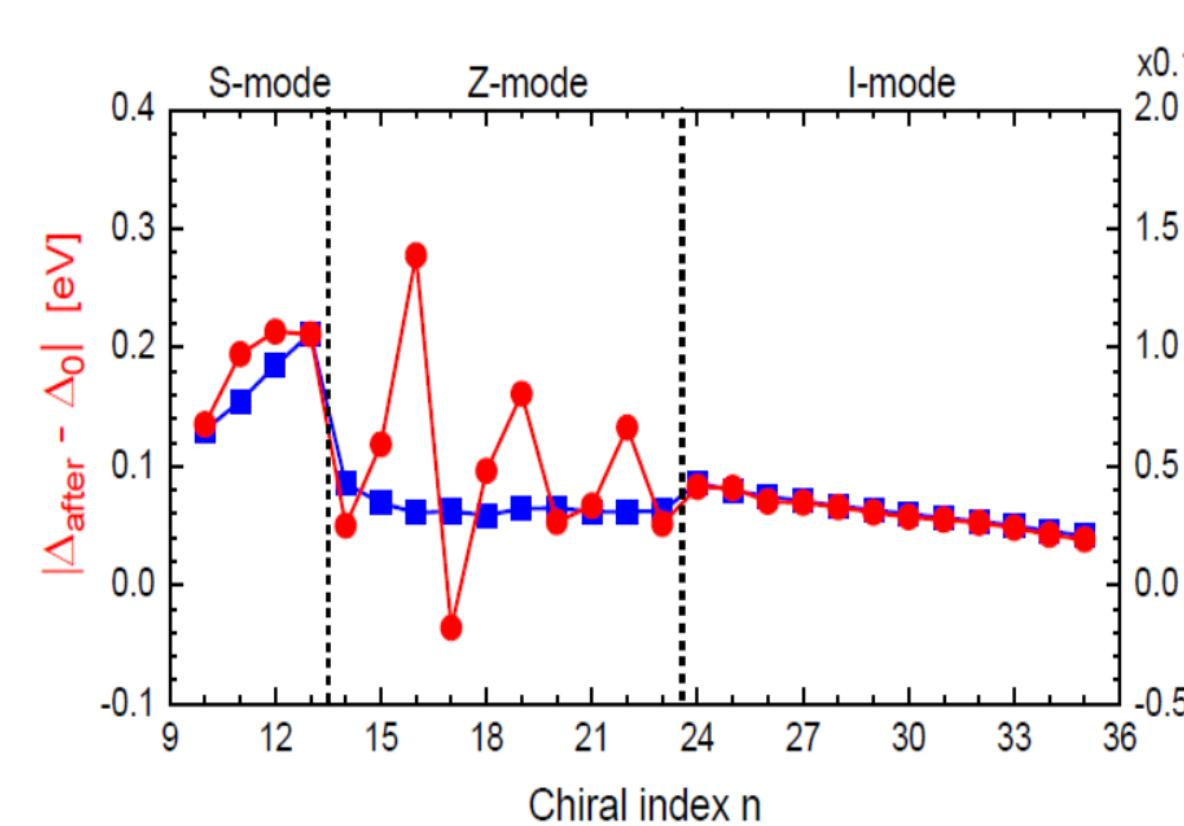
Nanotube diameter vs. buckling mode, buckling-induced band gap change, and post-buckling stress
