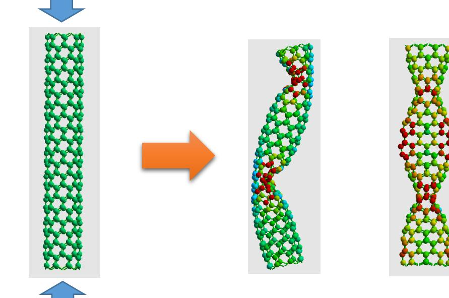
Atomistic model analysis of buckling behavior of carbon nanotubes under axial compression
