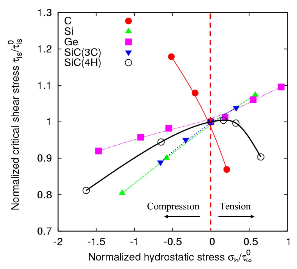
Ideal shear stress (ISS) under compression/tension in covalent crystals
