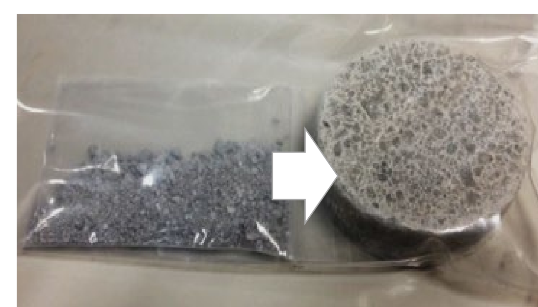
Recycling of crushed concrete
