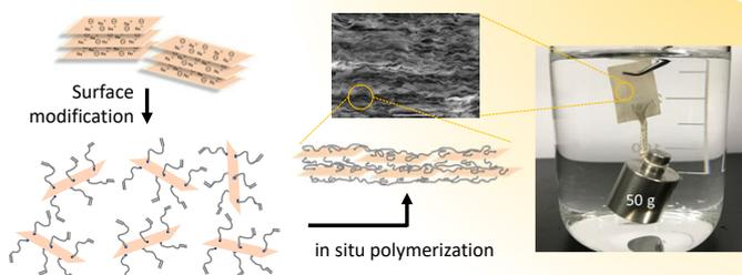
Nacre in sea shells is an organic/inorganic nanohybrid consisting of alternating layers of plate-like minerals and organic polymers and is known for its high rigidity and low permeability. However, artificial nacre-mimetic materials are often water-sensitive because of high hydrophilicity of the inorganic component. We developed a rigid, water-proof nanohybrid by combining the surface modification and in situ polymerization techniques.
