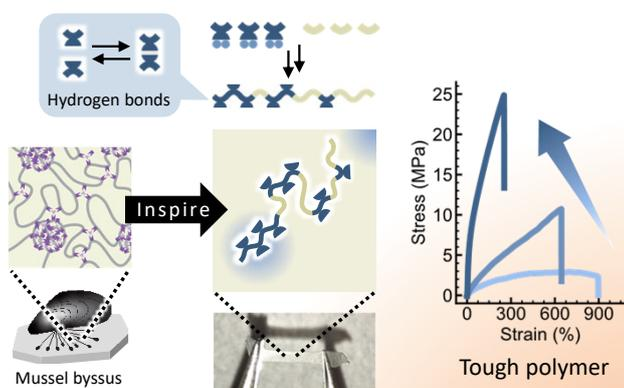
Mussels have a string-like tough organ called *byssus* to fix themselves to rocks. Inspired by the multiphase structure formed by dynamic crosslinks in byssus, we developed a new material with high mechanical toughness.
