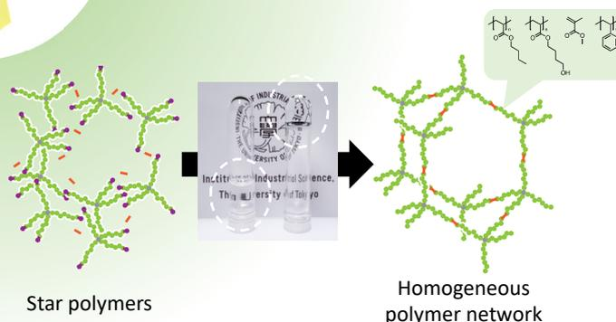
Elastic polymer materials such as rubbers and gels are made of numerous polymer chains cross-linked with each other, forming 3D-network. However, the network structure is usually highly heterogeneous, which has negative influences on the materials' performance. We developed a novel synthetic method to make highly homogeneous polymer networks.
