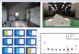
Experimental house natural ventilation prediction using 3 methods (field measurement, wind tunnel experiment, CFD simulation)
