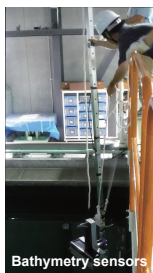
Fig4: Experiment of Multibeam-echosounder
