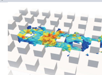
Computational prediction of pollutant dispersion in block-arrayed urban model
